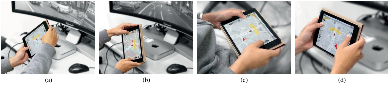
Fig. 4 MapXplorer interaction controls: (a) Motion gesture for left steering; (b) Motion gesture for right steering; (c) Side panning for moving forward or backward when device is laid down; (d) Side panning for pitching up or down the street view when device is stood up.
