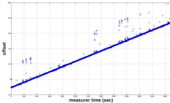
Fig. 1. A scatter diagram of 5000 offsets collected under wired network. The measurer's time is normalized by setting the receiving time of the first packet as 0 second. The values of offsets, in unit of millisecond, are also shifted such that the offset of the first packet is always 0.
