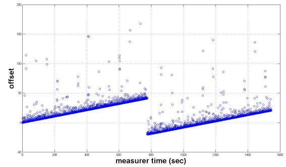
Fig. 3. A scatter diagram of 5000 offsets. The sender conducted a time synchronization during the measurement.
