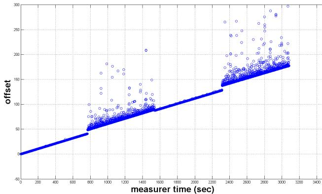
Fig. 2. A scatter diagram of 6000 offsets collected partially under wired network and partially under wireless network.
